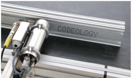
The i100 is a stainless steel, modular inkjet printer designed for ease of use and reliability in today's 24/7 factory environments. The i100 can print one or two lines of print on one or both sides of a product, on the top or even underneath. The MEK ink dries within seconds on any non-porous substrate. The ink system is totally sealed meaning that unlike continuous MEK ink jets there are no expensive makeup fluids or solvents to evaporate.
