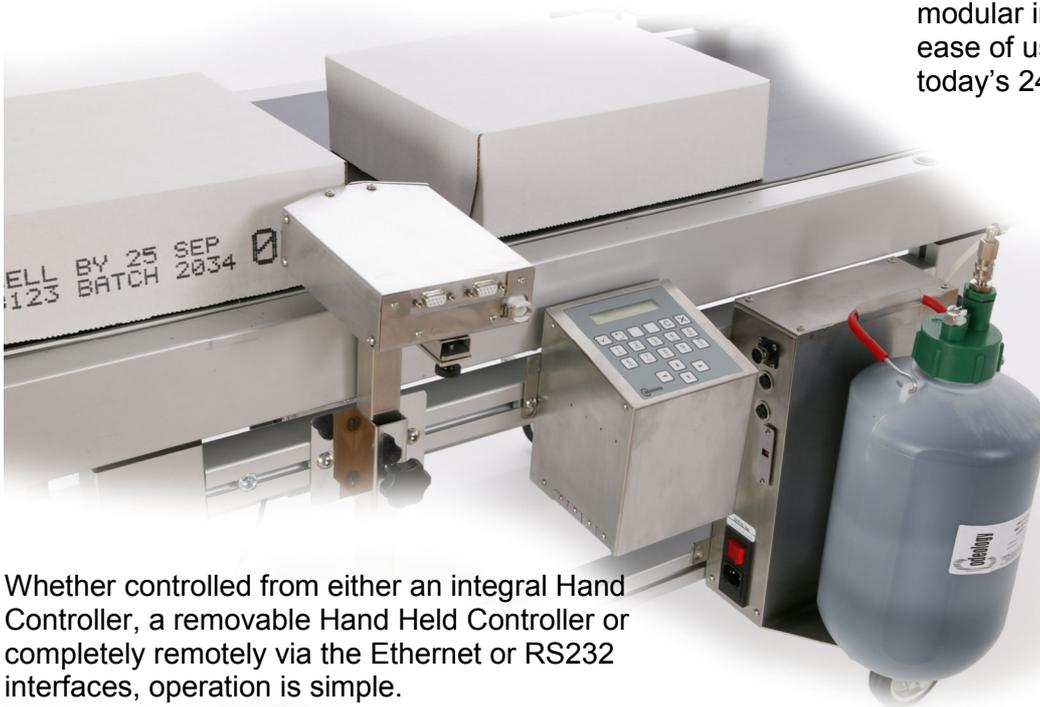
Whether controlled from either an integral Hand Controller, a removable Hand Held Controller or completely remotely via the Ethernet or RS232 interfaces, operation is simple.
