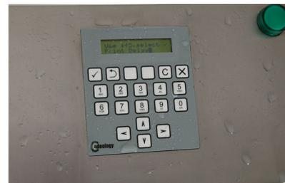
Print message editing uses the same method as mobile phone texting, allowing a small number of keys to call up the entire alphabet with ease. Training your operators to edit print messages is not difficult, as most operators are already comfortable with texting methods.
