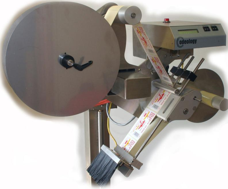
The P140 is a robust machine designed to apply labels simply and inexpensively. If you need to apply pre-printed labels to an accuracy of +/-5mm then why pay for more expensive machines with servo drives or stepper motors that give you more accuracy than you need? We use a proven dc motor that gives low cost label application without the expensive feedback or control mechanisms associated with more complex drive systems.
