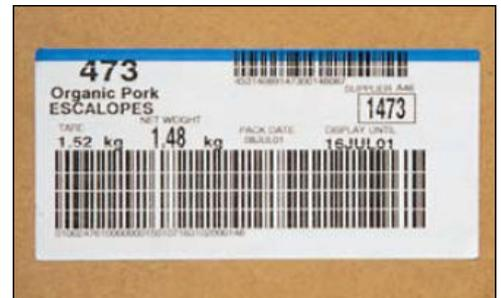
You have to look a little harder on this one. Notice that the label is applied in the wrong position so that the barcode wraps around the corner of the carton. This barcode will not read as the scanner will not be able to see all of the barcode on that face.
