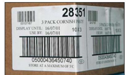
What about the third one? Although this one looks reasonably good with no horizontal lines and the quiet zones are wide, a verifier would reveal the problem. The dark bars on the barcode are too wide in relation to the gaps. This is caused by the temperature setting in the label design software set too high, and again this will not scan correctly.
