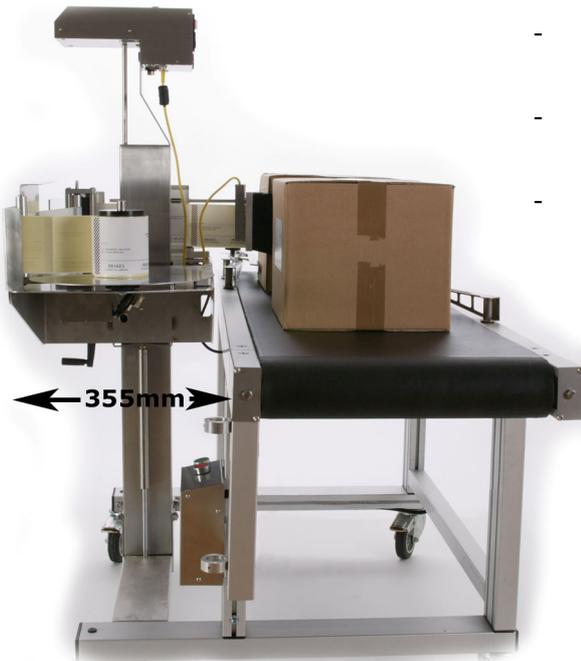
Options include integral conveyors, barcode scanners and barcode verifiers.
