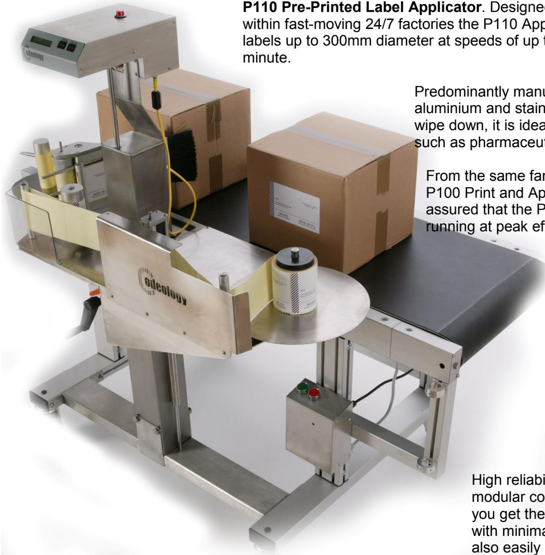
High reliability, easy setup and modular components ensure that you get the most out of the P110 with minimal intervention. It can also easily be upgraded to a full print and apply system by adding a print engine.
