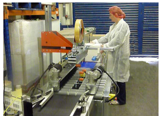
Products slid across and down into the cartons gives much higher throughput and less operator strain than Lazy Susans.
